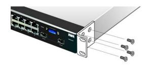
Figure 3-2: Attach the Brackets to the Switch
